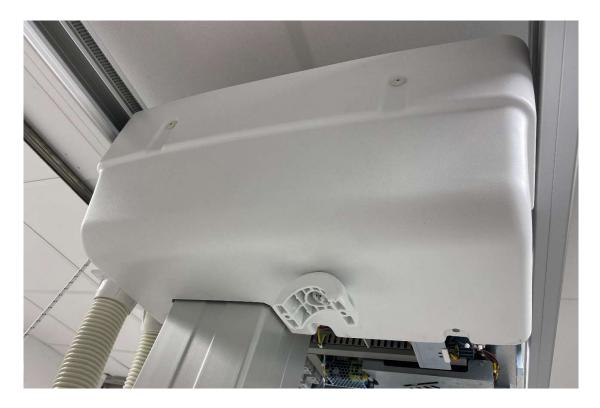
21. Hang the cable back up and reattach the two Torx T20 screws for the cable holder.
