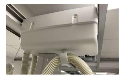
22. Re-mount the right-hand cover of the ceiling wagon using the two screws.
