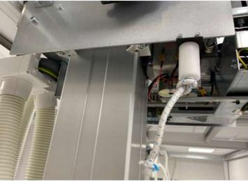
11. Release the screw holding electrical plate 1.1 and fold down the plate on its hinges. **NOTE!** Support the electrical plate during this step to prevent it from falling.
