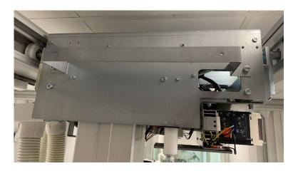
13. Release the two screws enough to slide on the receiver bracket, p/n 0073-007-208 from the upgrade kit.
