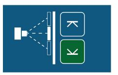
Collimate to the upper border and press the upper arrow key (turns green).
