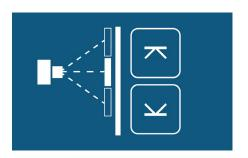
Collimate to the lower border and select the lower arrow key (turns green).
