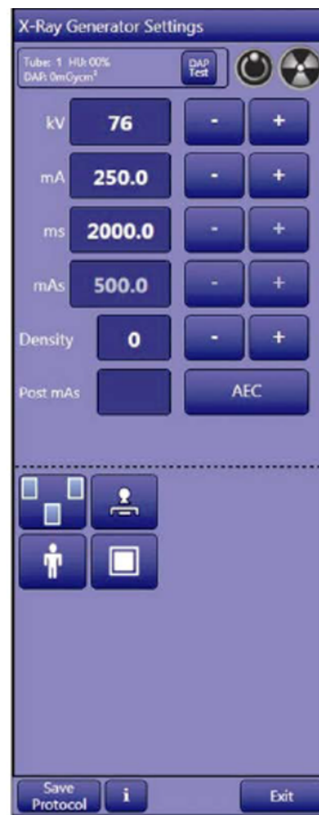
Control panel, AEC mode
