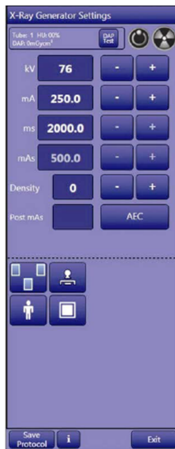
Control panel, AEC mode
