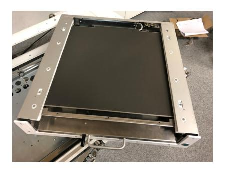
NOTE! Be very careful when handling this – the AEC-chamber is highly sensitive, even minor bending and tweaking could damage it.
