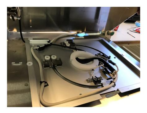
NOTE! Make sure that the cable is not interfering with any of the microswitches.
