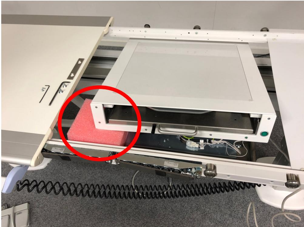
**NOTE!** Be careful when lifting and angling the bucky not to scratch the cover surfaces.
