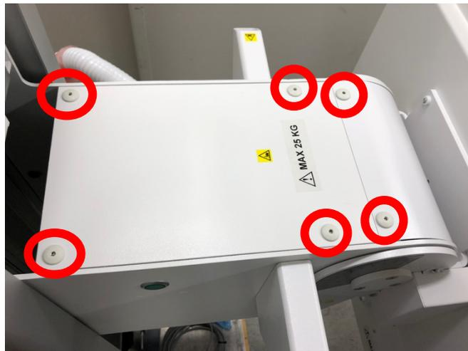
**1.4.7** Remove the cover between bucky attachment plate and bucky wagon:
