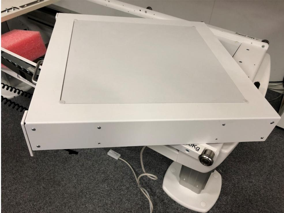
**1.5.9** Remove the screws and lift the cover off upwards:
