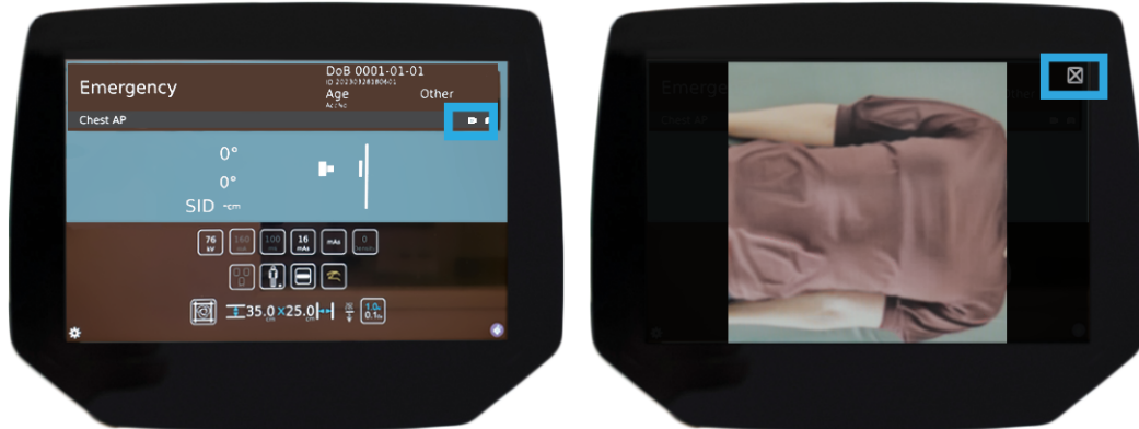
Fig. 3-47 Live camera displayed on the OTC. Press the camera icon (left) to activate, and close it by selecting the button in the upper-right corner (right).
