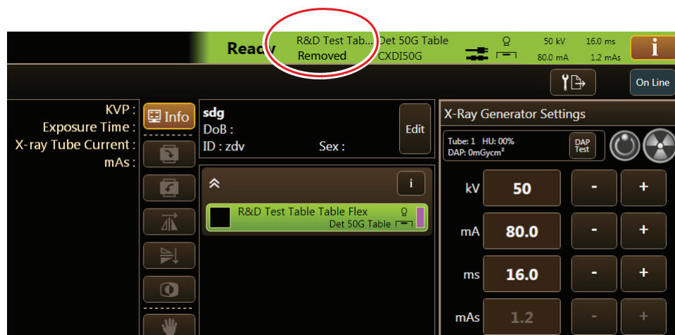
Fig. 3-45 Canon NE user interface. Grid removed.
