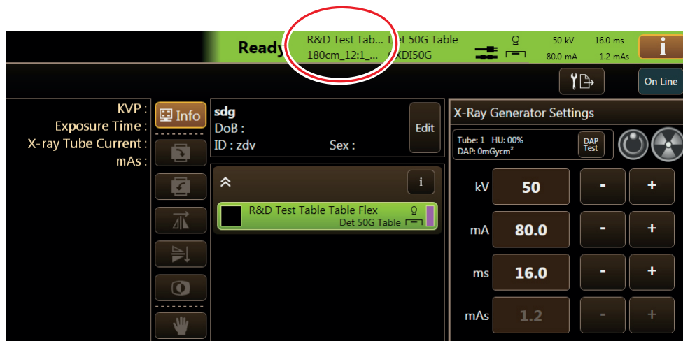
Fig. 3-44 Canon NE user interface. Grid data displayed.
