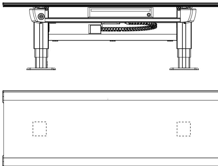
*Fig. 2-7 Placement of the table top when loading the patient.*
