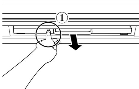
Fig. 4-40 Releasing the detector tray
