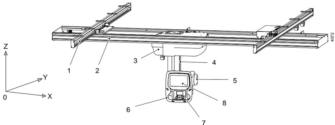
Fig. 1-3 Overhead Tube Crane, OTC
