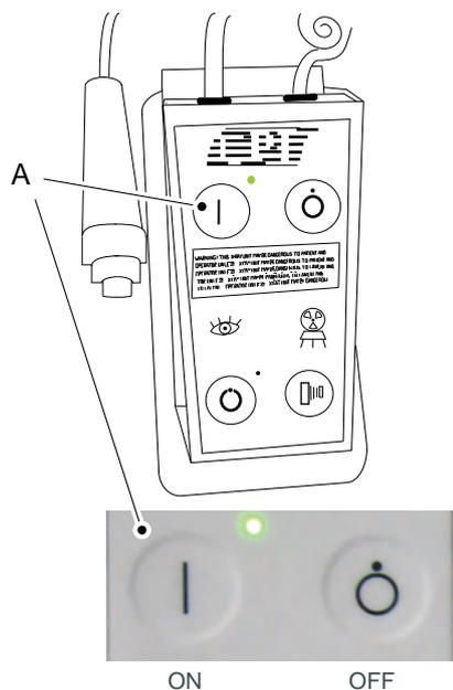
1. Press the power [ON] button (A) on the mini console.
