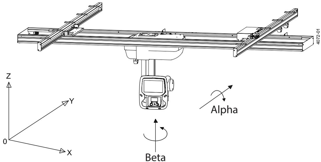
Fig. 3-1 OTC direction of movement
