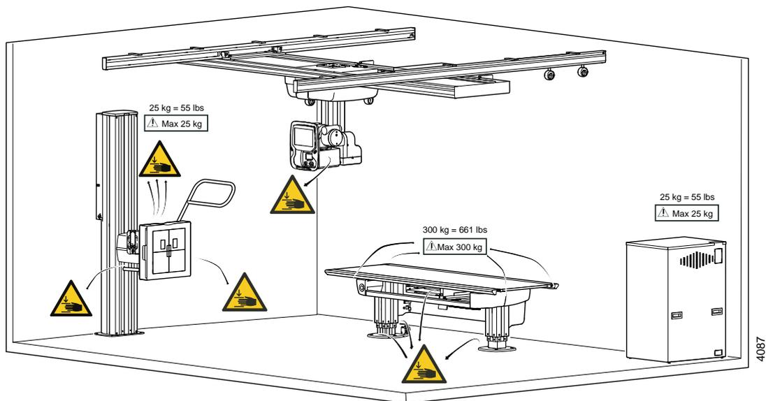
Fig. 2-1 Locations of safety and warning labels
