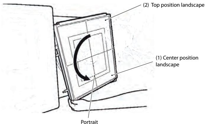
Fig. 4-37 Rotating the detector
