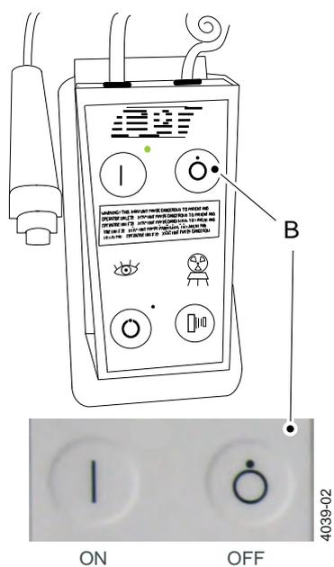
4. Press the power [OFF] button (B) on the mini console.
