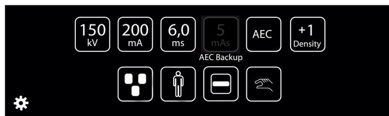
Fig. 3-25 mAs selection button grayed out
