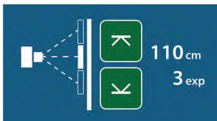
Fig. 4-36 Stitching mode — upper and lower limit set
