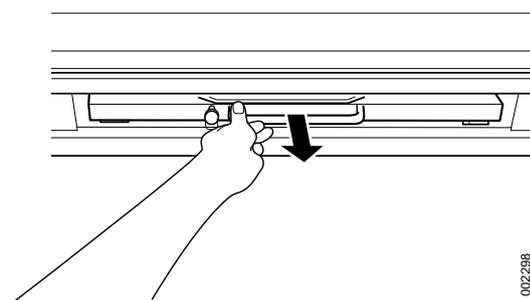
Fig. 4-49 Pull out the grid
