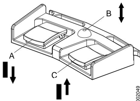
Fig. 3-50 Wallstand foot control manoeuvring
