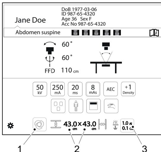
1. Select *Automatic* or *Manual* mode of the collimator.
