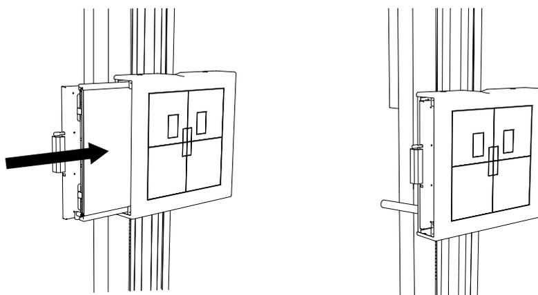
4. Push the detector until the hold-backs are set. Then the detector is in the correct position. Chargeable detectors will start charging when set in this position.
