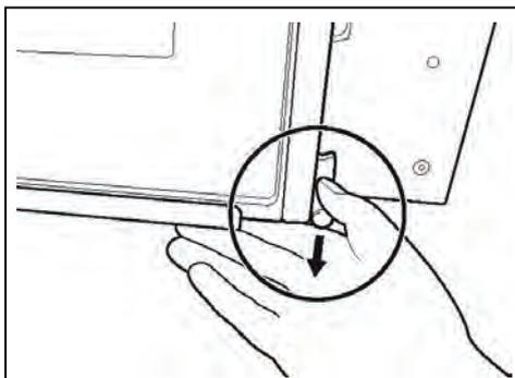
*Fig. 4-38 Unlocking the detector latch*
