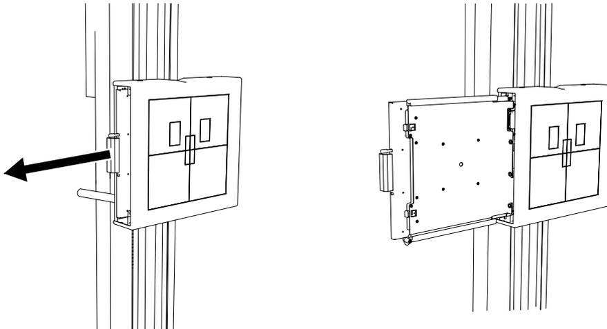
2. Insert the detector into the detector tray as shown below and set it by pushing the detector, holding down the latch.
