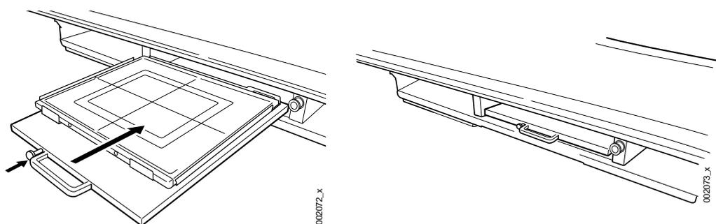
Fig. 4-44 Reinserting the detector tray
