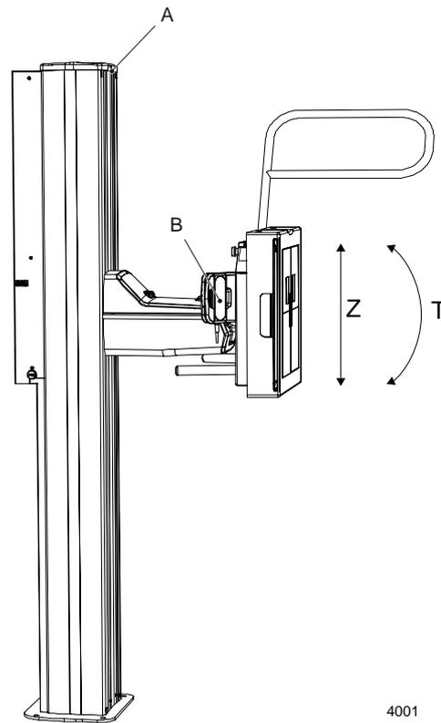
*Fig. 3-48 Wall stand, direction of movement*
