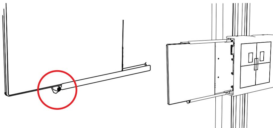
3. While pressing and holding the button of the detector tray, return it back to the inside of the detector holder.
