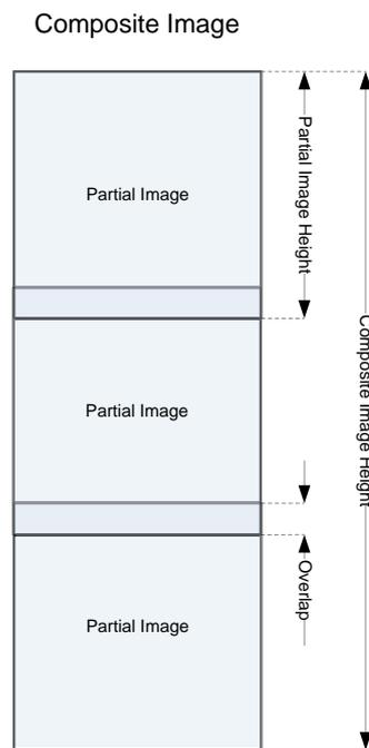
*Fig. 3-33 Stitching, schematic description*
