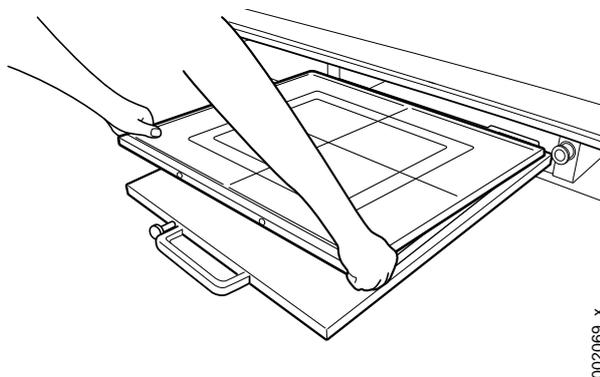
Fig. 4-42 Inserting the detector into the detector tray
