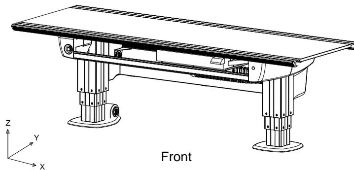
*Fig. 3-37 Directions of movement, Table*
