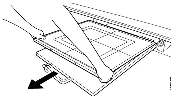
Fig. 4-48 *Detector removal*
