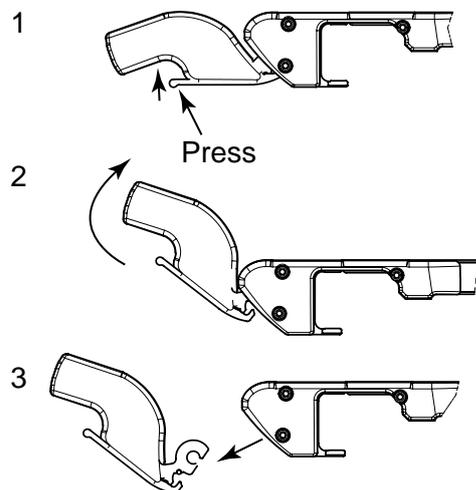
*Fig. 3-47 Removing accessories*
