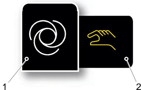
In automatic mode, the collimator light height and width is set from the anatomical program. The collimator light size can still be changed manually. In manual mode the collimator light height and width is not set from the anatomical program.
