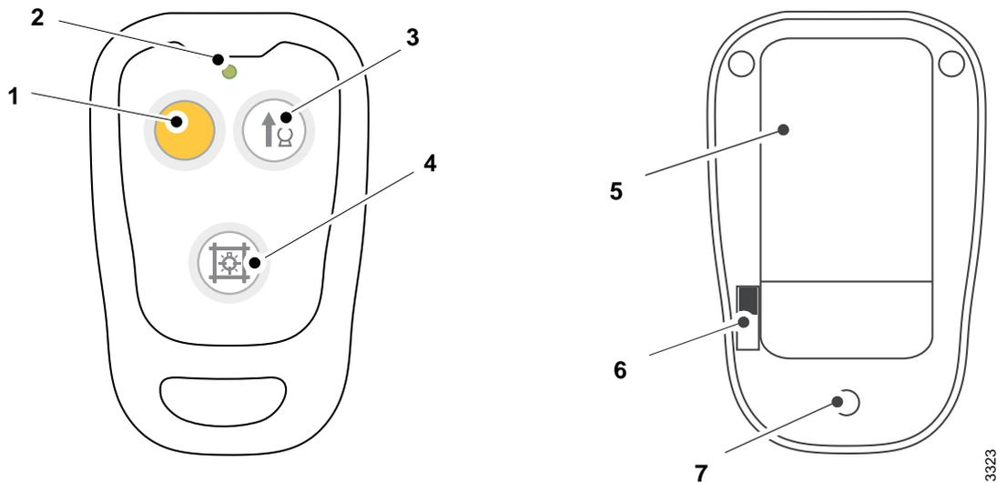
Fig. 3-35 Remote control, front and back
