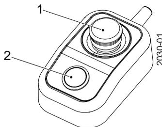
Fig. 3-36 External servo button module
