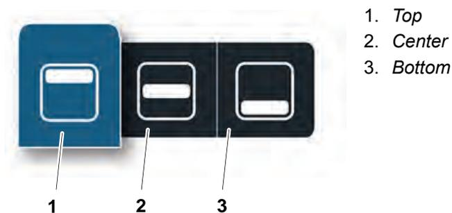
Fig. 3-29 Collimator centering selection
