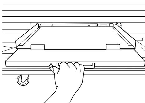
Fig. 4-41 Pulling out the detector tray
