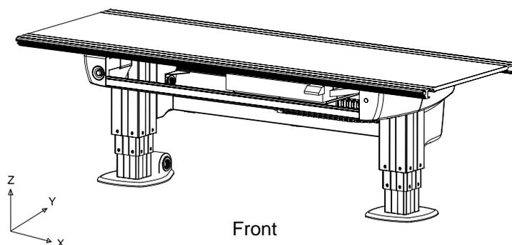
Fig. 3-45 Directions of movement, Table
