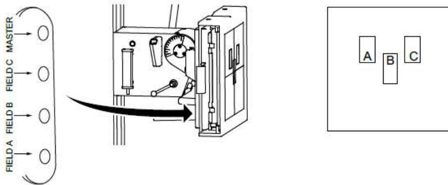
7. Select the Left-side AEC Field and repeat step 2-6 until target EI, is achieved. Adjustments are made on the potentiometer for the Left field.
