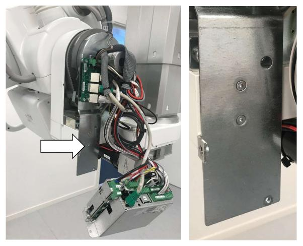
5. Turn away the board bracket to gain access to the alpha brake magnet.
