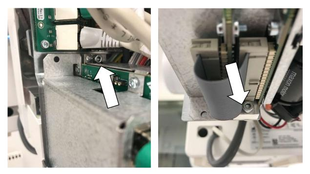
4. Release and remove the two screws for the board bracket.
