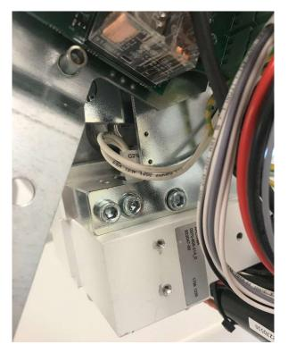
6. Release the two screws for the magnet brake bracket.
