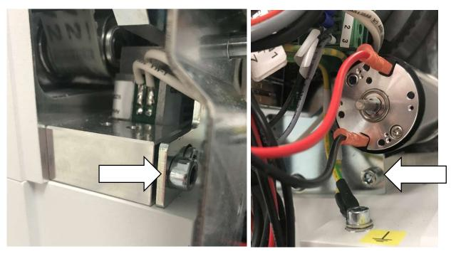
7. Remove one of the screws and slide in shim washers to create clearance between brake magnet and brake plate. The amount of shims needed depends on the situation but a good starting point is 0,2mm.
