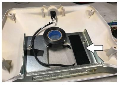
Using one of these two measures, or both, will prevent shortcuts on the 24V line and the error message from appearing.
