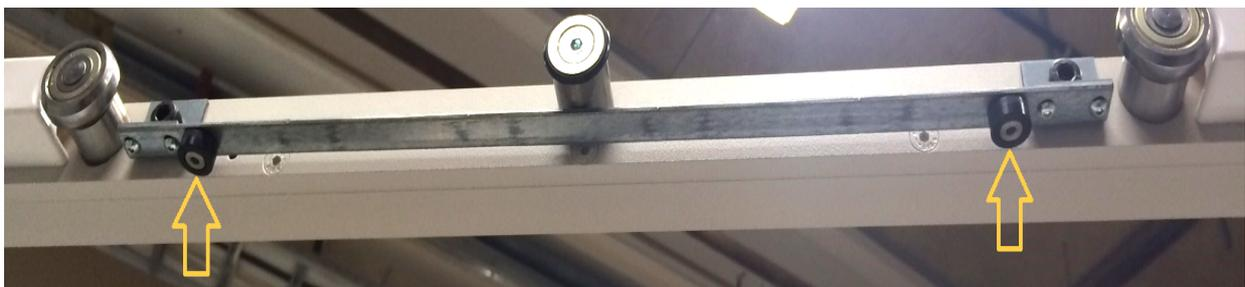
7. The black wheels must be adjusted so that they are easily turned by hand. If adjusted too tight the table top will not run smoothly.
