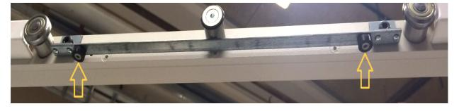
7. The black wheels must be adjusted so that they are easily turned by hand. If adjusted too tight the table top will not run smoothly.
