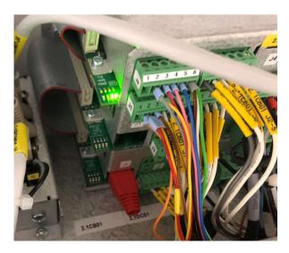
CB01 LEDS: D1=OFF, D2=OFF, D3=FLASHING, D4=ON
