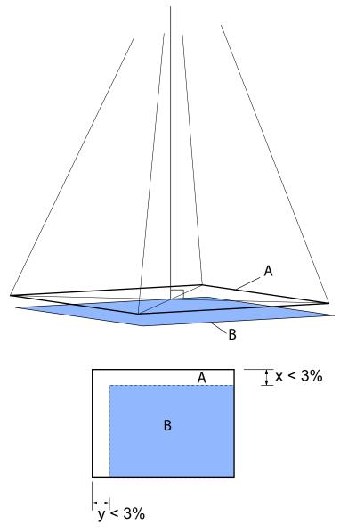
Fig. 4-118 X-ray field and Image reception area
