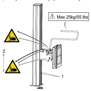
Fig. 2-18 Possible squeeze hazards
