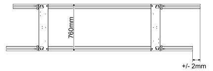
Fig. 4-7 Distance between traverse rails X
