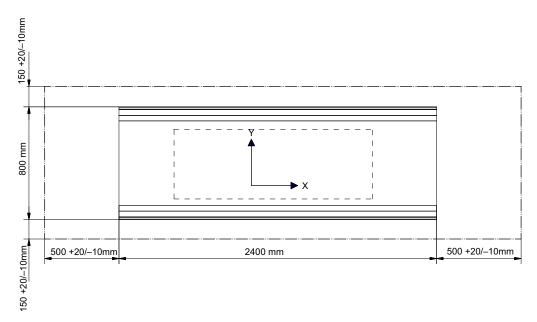
Fig. 2-13 Stroke length
