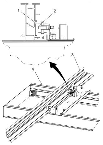
Fig. 4-13 Installing the Y brakes
