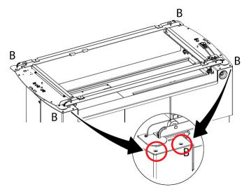
Fig. 4-82 Remove the 8 screws at "B"
