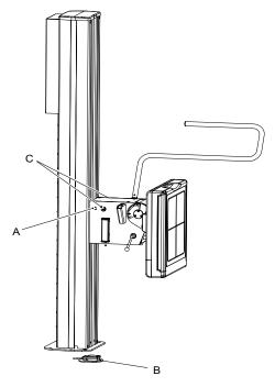
Fig. 3-12 Motorized Z-movement controls
