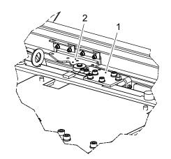
1. Place the positioning index (2) in position next to the index positioning arm (1).
