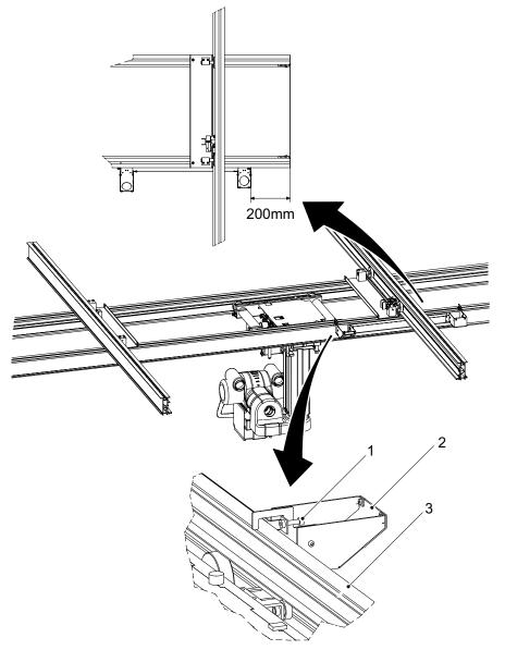
Fig. 4-21 Installing cable channel
