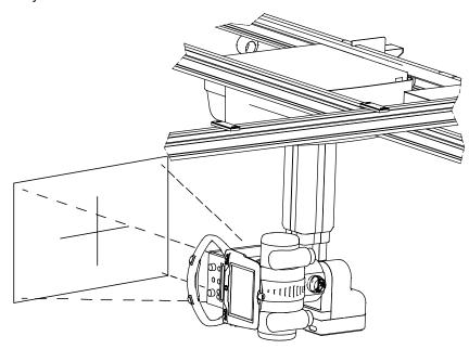
Fig. 4-58 OTC vertical alignment
