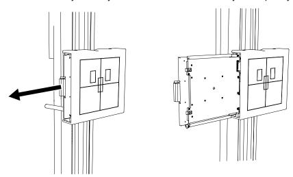
Fig. 3-16 Pull out detector tray
