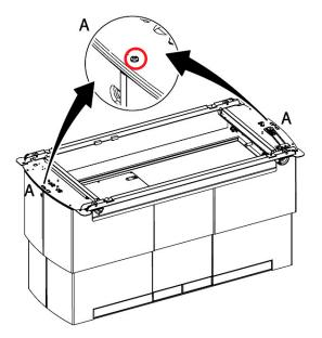
Fig. 4-81 Remove the 2 screws at "A"
