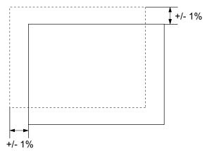
Fig. 4-115 Collimator light and X-ray field alignment
