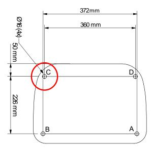
Fig. 4-71 Marking template Wallstand (Isolation plate)
