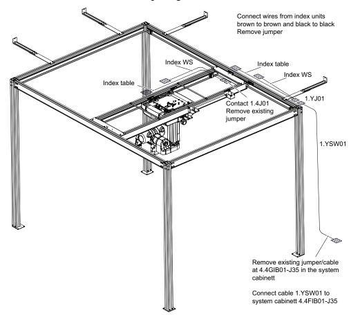
Fig. 4-130 Connecting electrical indexes
