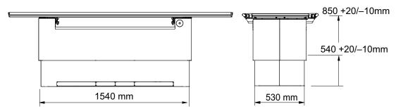
Fig. 2-14 Dimensions underneath the Table
