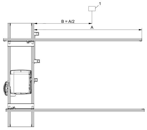
Fig. 4-24 Installing wall attachment
