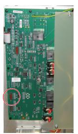
Fig. 4-47 480V, DIP switch SW3-8
