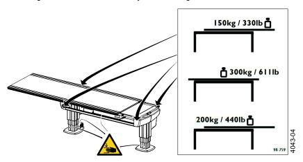
Fig. 2-2 Location of the weight restriction labels and warning labels, table 0055
