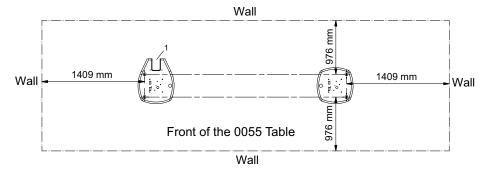
Fig. 4-95 Necessary space, table movement
