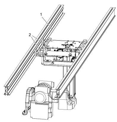
Fig. 4-9 Brake steel bars
