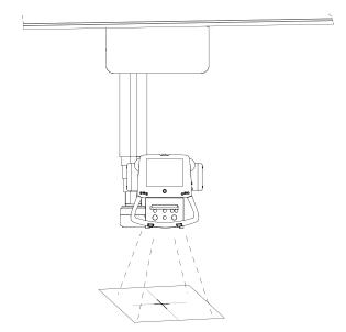
Fig. 4-60 OTC horizontal alignment
