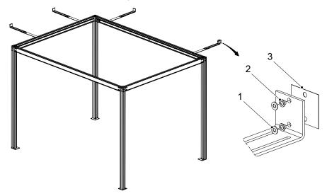
Fig. 10-6 Installing into the wall
