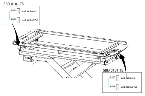
Fig. 4-93 Hand control attachment
