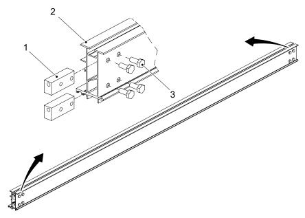
Fig. 10-1 Installing brackets
