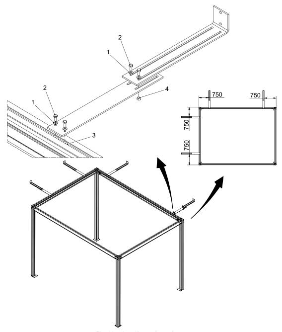
Fig. 10-4 Installing wall attachment
