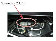
Power cable connected to connector 2.1J01
