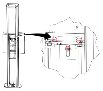
Fig. 4-69 Removing locking device
