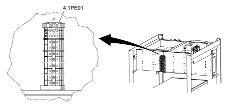
Fig. 4-110 Measuring protective earth
