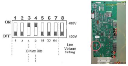
Fig. 4-37 400V, DIP switch SW3-8
