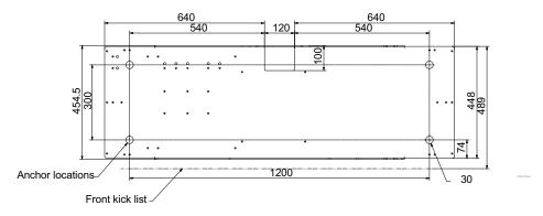
Fig. 4-87 Measurements for the Table bottom plate
