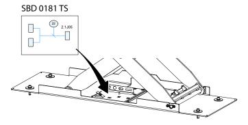
Fig. 4-92 Foot pedal attachment
