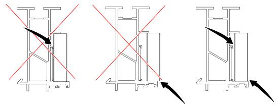
Fig. 4-11 Mounting of wheels
