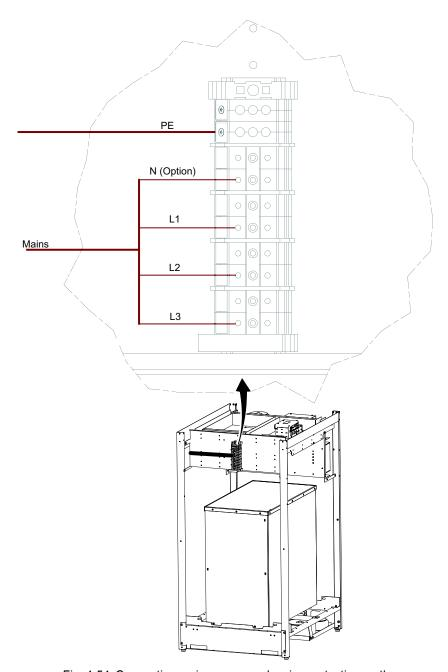
Fig. 4-54 Connecting mains power and mains protective earth
