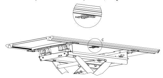
Fig. 4-102 Table mechanical stops
