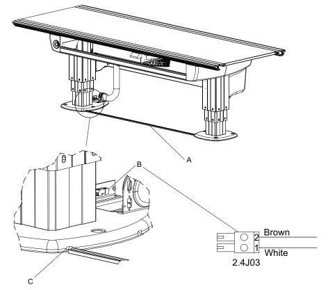
Fig. 4-108 Connect the foot control X/Y
