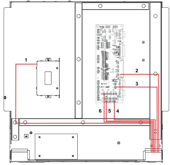
Wiring to electrical plate 4.4 is made in accordance with cable path 3, see Fig. 4-29.
