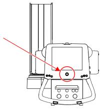
Fig. 3-25 Synchronization button with indication light — display
