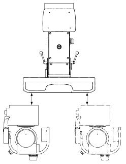
Fig. 4-70 Alignment of Wallstand
