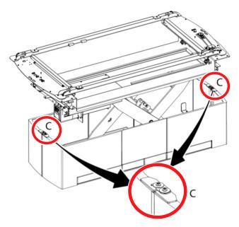
Fig. 4-84 Front screw of lower cover
