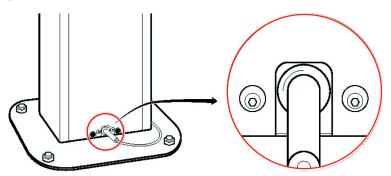
Fig. 4-66 Removing the two screws at the Wallstand back
