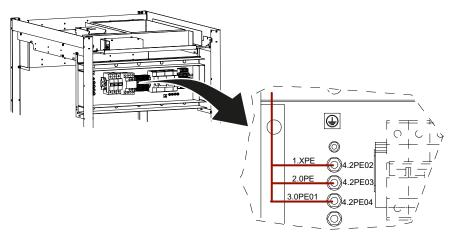
Fig. 4-109 Checking the protective earth cables and bolts
