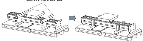
Fig. 4-62 Removing cross-ties
