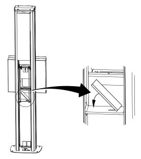
Fig. 4-68 Installing counterweights
