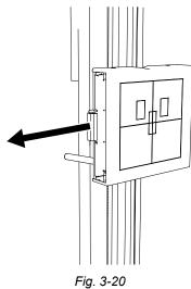
2. Hold down the latch, removing the detector from the detector tray as shown below.
