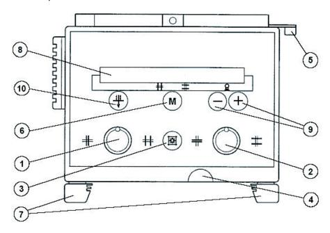
Fig. 3-3 Siemens AL02 Collimator Controls
