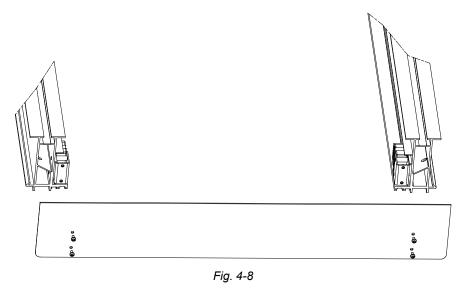
Before installing the traverse rails X, check that the steel bar for the brakes is placed in the correct traverse rail X.
