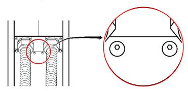
Fig. 4-74 Reassembling the two screws under the electrical box
