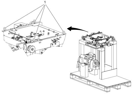
Fig. 4-14 Lifting ceiling wagon
