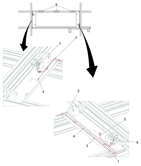
Fig. 4-22 Connecting cables to Y-brakes
