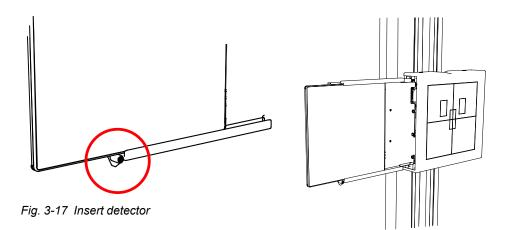
3. While pressing and holding the button of the detector tray, return it back to the inside of the detector holder.
