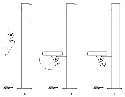
Fig. 3-14 Tilting detector holder
