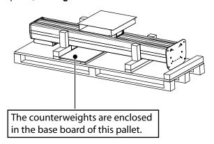
Fig. 4-63 Lifting Wallstand off the pallet
