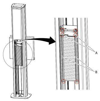
Fig. 4-67 Loosen screws
