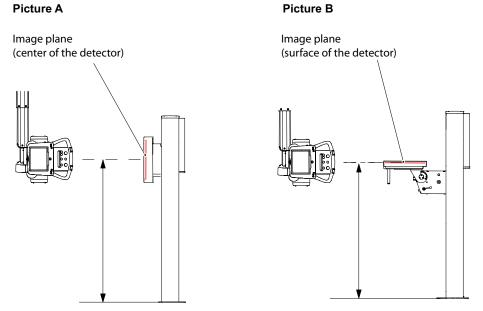
Fig. 4-146 Measuring the height
