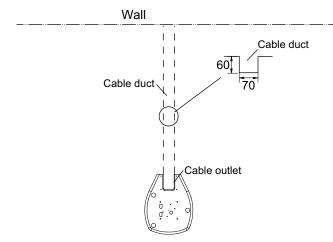
Fig. 4-96 Cable duct in the floor
