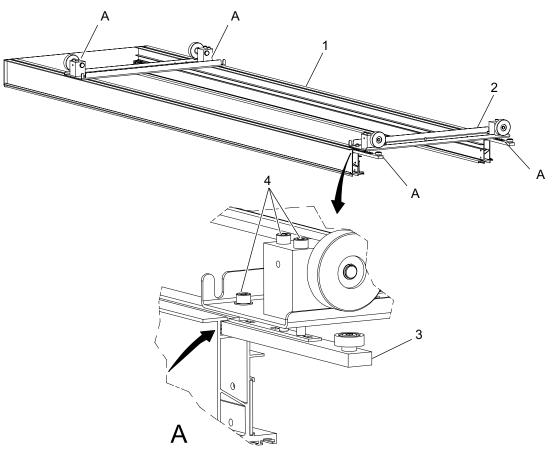
Fig. 4-6 Traverse rails X
