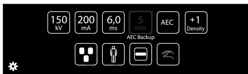
Fig. 3-5 mAs selection button grayed out
